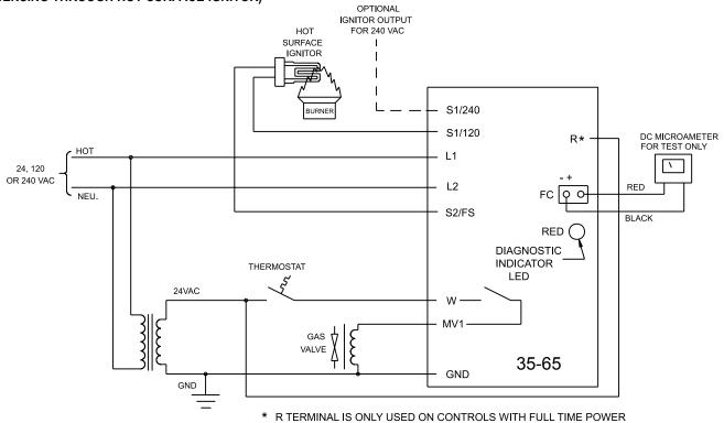
REMOTE FLAME SENSING (SENSING THROUGH INDEPENDENT FLAME ROD)
