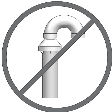
Figure 4-5 Do Not Install U-Bent to Rain Cap
