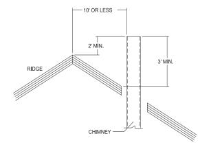
Figure 10 - Vent Termination from Peaked Roof - 10' or Less From Ridge
