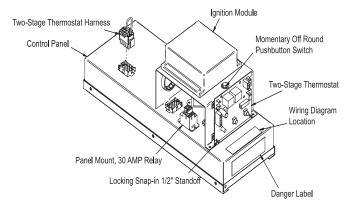
Figure 23A - Models 495,000 - 745,000 Btu/hr Control Panel Component Location Drawing
