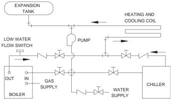
Figure 29 - Installation with a Chilled Water System
