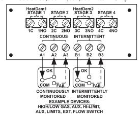
Figure 24D - Field-Installed Safety Devices - Models 985,000 - 2,065,000 Btu/hr Only
