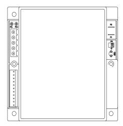
Figure 39 - Hot Surface Ignition Control Module
