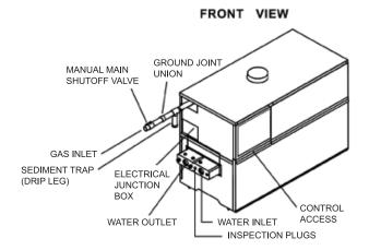
Figure 17 - 495,000 - 745,000 Btu/hr Gas Line Connection Example
