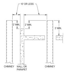
Figure 12 - Vent Termination from Flat Roof 10' or Less from Parapet Wall
