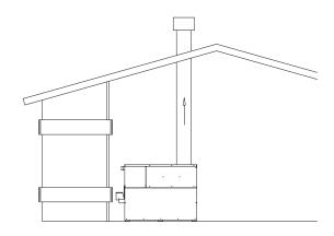
**Figure 8 - Outside Combustion Air Through Ducts**
