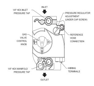
Figure 33 - Combination Gas Valve
