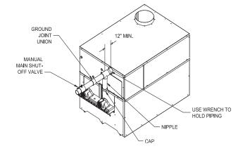
Figure 18 - 985,000 - 2,065,000 Btu/hr Gas Line Connection Example
