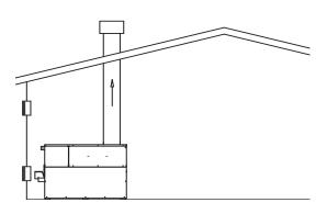
Figure 7 - Outside Combustion Air - Two Openings
