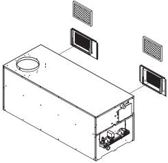
Figure 5 - Installing Combustion Air Filters, 1,795,000 and 2,065,000 Btu/hr Models
