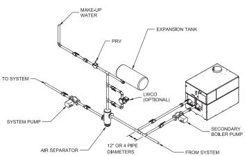
Figure 26 - Primary/Secondary Piping of a Single Boiler
