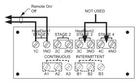
Figure 24B - Remote On/Off Boiler or Water Heater - Models 985,000 - 2,065,000 Btu/hr Only
