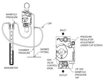
Figure 21 - Measuring Manifold Gas Pressure
