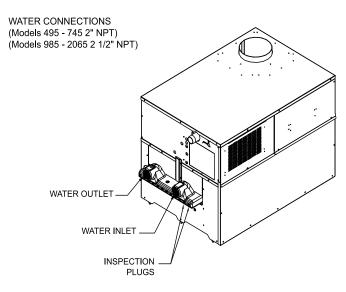
Figure 22 - Water Connections
