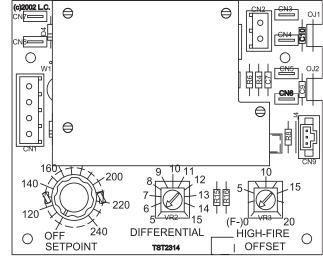
Figure 35 - Temperature Control Setting Knobs
