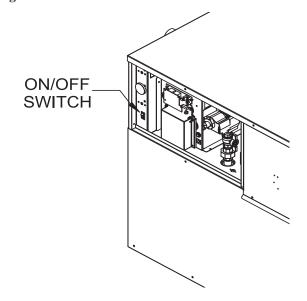
Figure 32 - ON/OFF Switch
