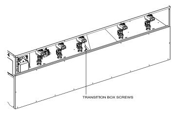
Figure 46 - Loosening the Transition Box Screws, 1,435,000, 1,795,000 and 2,065,000 Btu/hr Models Only
