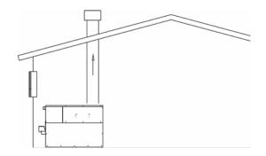
Figure 6 - Outside Combustion Air - Single Opening
