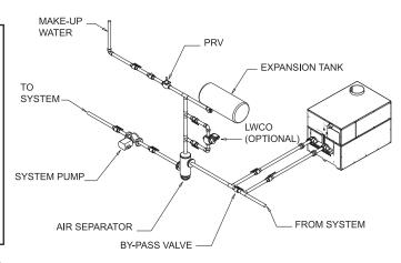
Figure 30 - Boiler Bypass Piping for High Flow Systems
