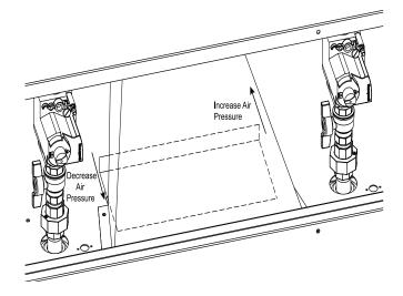
Figure 47 - Adjusting Air Shutter
