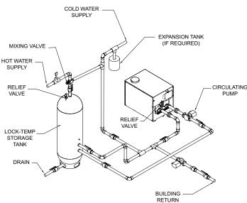
Figure 41 - Typical Water Heater Piping with Storage Tank
