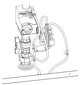
Figure 43 - Air Pressure Switch
