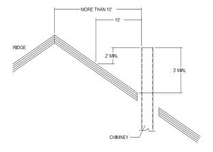
Figure 11 - Vent Termination from Peaked Roof More Than 10' From Ridge
