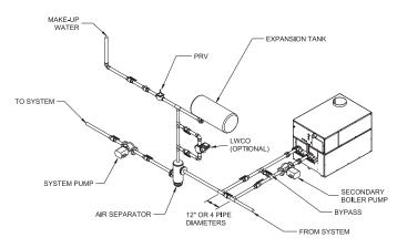
Figure 28 - Boiler with Low Temperature Bypass Piping
