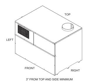
Figure 2 - Clearances from Combustible Construction
