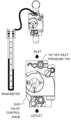
Figure 20 - Measuring Gas Supply Pressure at Combination Gas Valve
