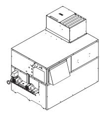
Figure 15 - Outdoor Vent Cap Installed on 495,000 - 1,435,000 Btu/hr Models
