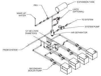
Figure 27 - Primary/Secondary Piping of Multiple Boilers
