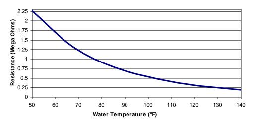
Figure 18-2 Thermistor Resistance Chart – 1 MOhm Water Probe (High Temp.)
