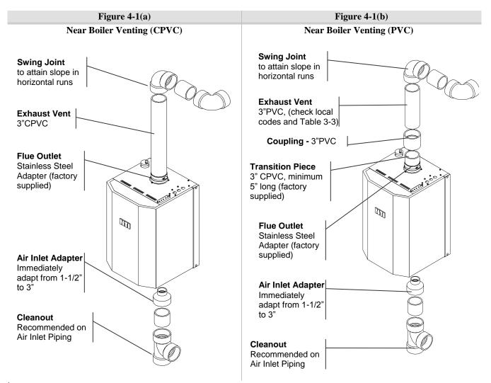
**<sup>★</sup> Air-Inlet** - check with applicable local codes for acceptable pipe material.
