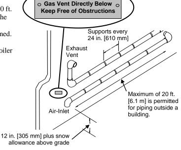
Figure 4-8 Existing Chimney Chase Way
