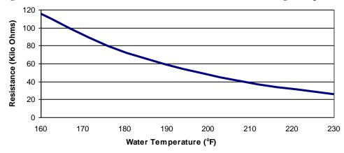
Figure 18-3 Thermistor Resistance Chart - 10 kOhm Outdoor Sensor
